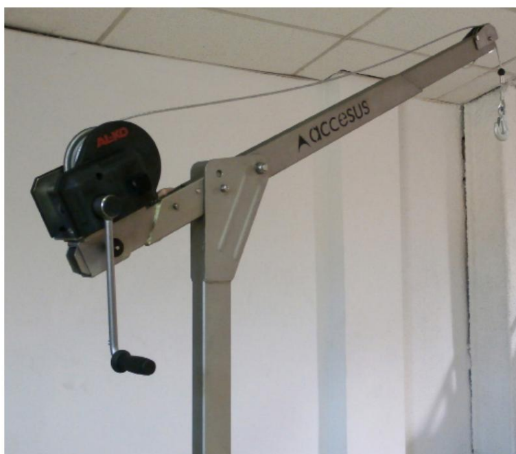
BR3 rescue arm with winch for loads
