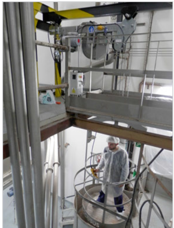
APPLICATION DESCENT EQUIPMENT AVAHO-S WITH CIRCULAR CRADLE Ø 1 METER IN AN INDUSTRIAL HOPPER
