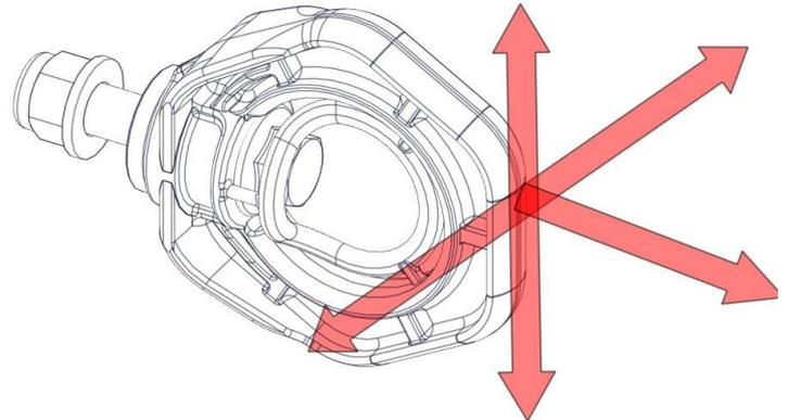
**Figure 1. Acceptable methods of installation of device**
