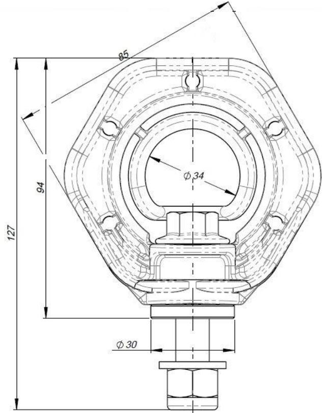
**Figure 2. Overall dimensions PAF185**
