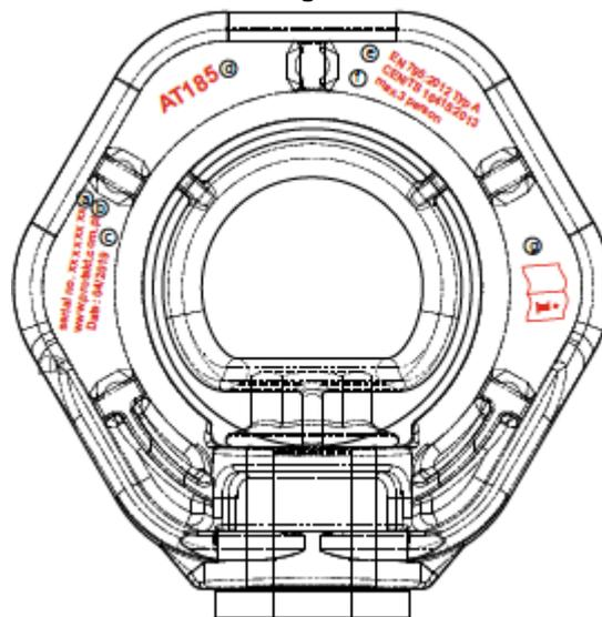
Figure 3. Method of device marking
