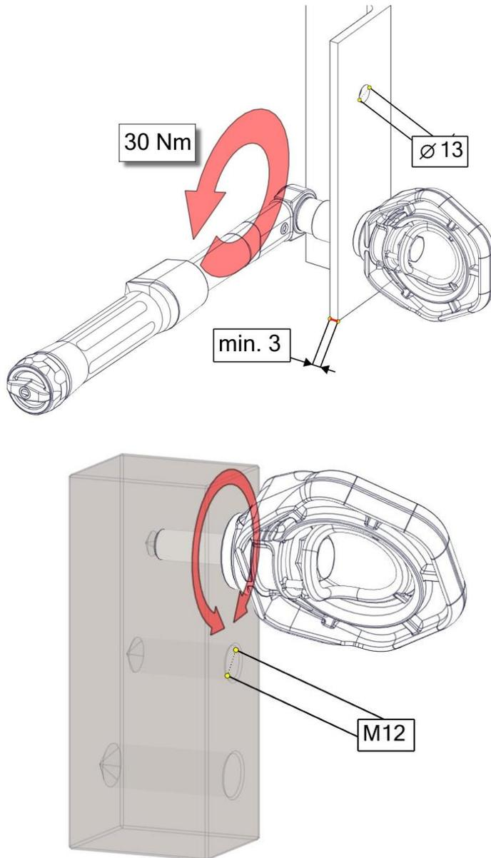
**Figure 4. Installation of anchor point**
