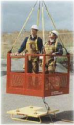
Work platform lifted by a crane using a sling (lifting accessory)
