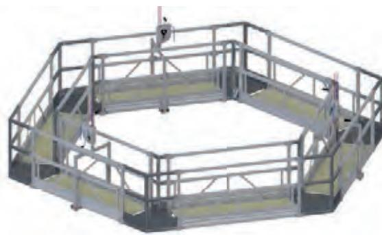
Platform made of 2 m length modules and 60° corner sections with 3 manual hoists and intermediate stirrups.
