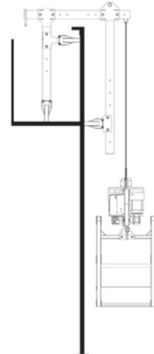
Suspension clamp for tank with floating roof
