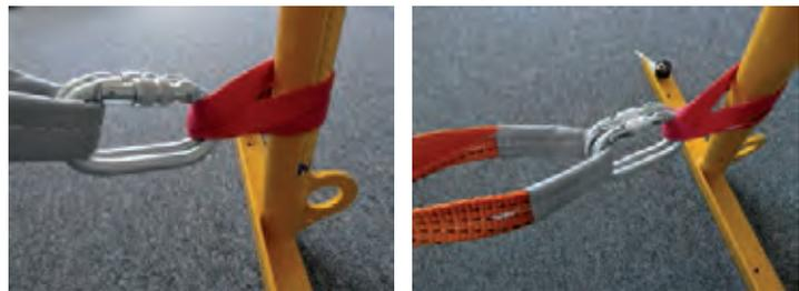
\* In case of the PAT 900 anchorage point, it must be mounted in a double way as shown in these photographs.
