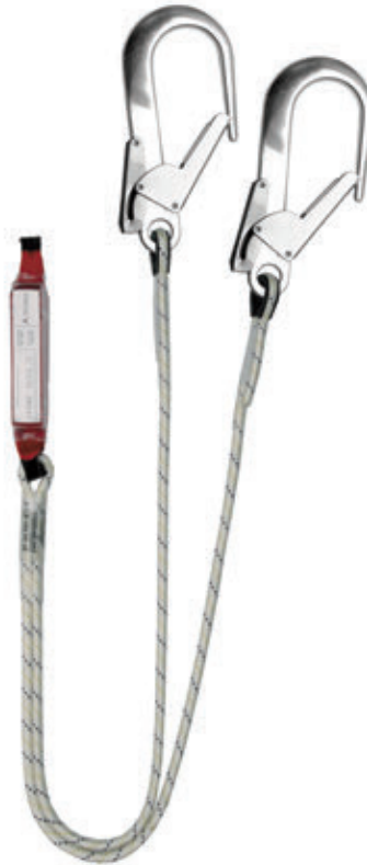
Ref. ABE+2ES102(C) Double lanyard of 2 m in length, with two AA023 aluminium hooks and Ø60mm aperture
