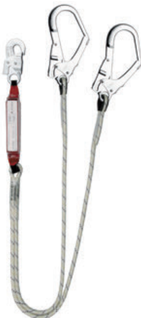
Ref. ABE+2ES102(F) Double lanyard of 2 m in length, with two aluminium AA023 and Ø60mm aperture + AA002 hook
