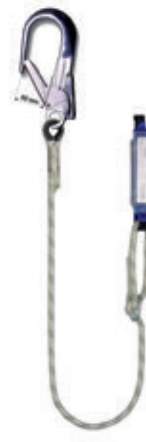
Ref. ABE+ES100(C) Adjustable single sling with absorber, 2 m in length, with AA023 aluminium hook and Ø60mm aperture.
