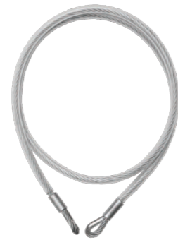
PAC 410 Steel sling with 8 mm grommets to connect with a carabiner. 15 kN and 3 available lengths: 0.5, 1 and 2 m.
