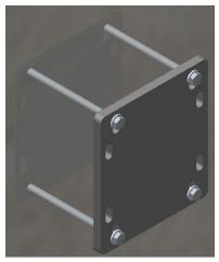
2- We will then drill the 4 **holes on the slab with a 14 mm diameter drill bit**. It is very important to carry out this operation keeping the holes perpendicular to the face of the slab.
