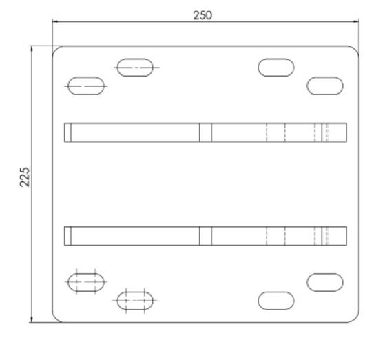
The weight of the plate with clamping ears is 9.5 kg.
