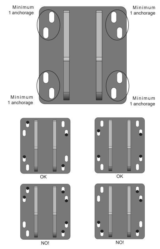
It is forbidden to use the plate if the above-mentioned anchors are not installed.
