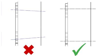
3- Finally we will center the plate on the opposite side of the slab with respect to the holes made and we will fix it to the counterplate thanks to its threaded rods with a torque of 62 Nm.
