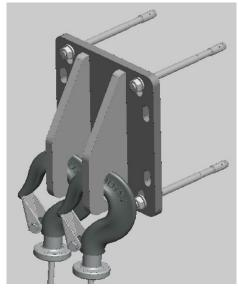
2- Using 4 Hilti® HAS M12x110/28 **chemical anchorage** with HIT HY50 chemical cartridge or equivalent
