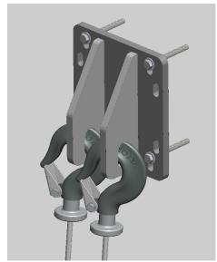
3- With counterplate and 4 threaded rods M12, minimum quality 8.8, together with their corresponding washers DIN125 and safety nuts DIN985 in. To do this, we will drill the 4 holes through which the threaded rods will pass and we will place the counterplate on the other side of the slab to sew the assembly.
